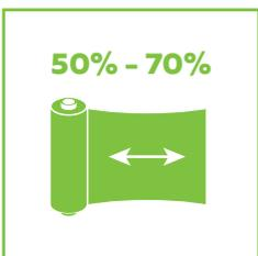
The recommended stretch of the film is 50% - 70%. To check the correct stretch, mark 2 points on the reel of film at a distance of 10 cm, after passing through the stretching rollers on the wrapping machine, the points should be 15 to 17 cm apart. To ensure optimum stretch, the machine rollers should be inspected and cleaned regularly.
