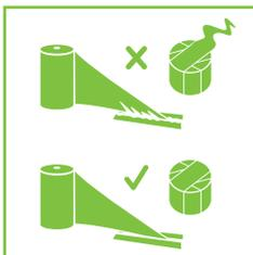
Special attention must be paid to the sharpness and condition of the cutting knives to ensure good adhesion of the film and to eliminate long film tails.
